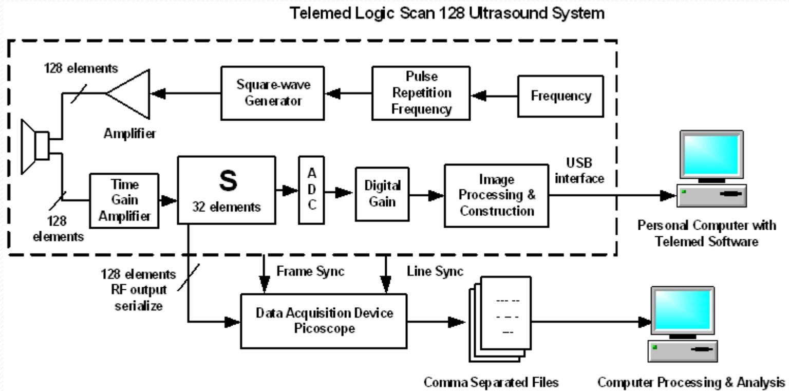
Figure 1. Experiment Setup
